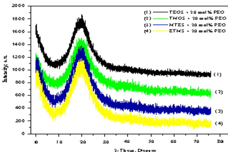
Fig.1. XRD patterns of nanomaterials containing PEO
