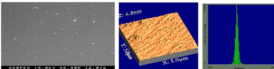
**Fig.4.** SEM, AFM image and roughness analysis of the hybrids with TEOS containing 20 % PEO
