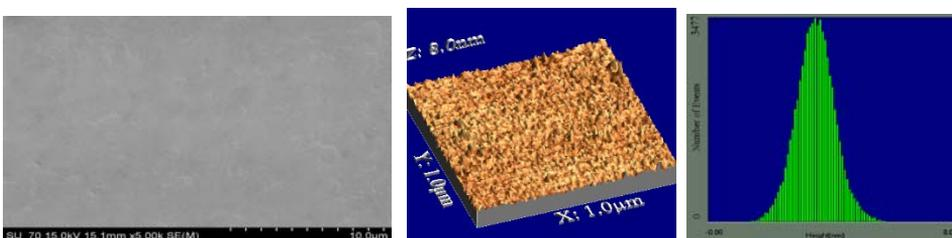
**Fig.6.** SEM, AFM image and roughness analysis of the hybrids with MTES containing 20 % PEO
