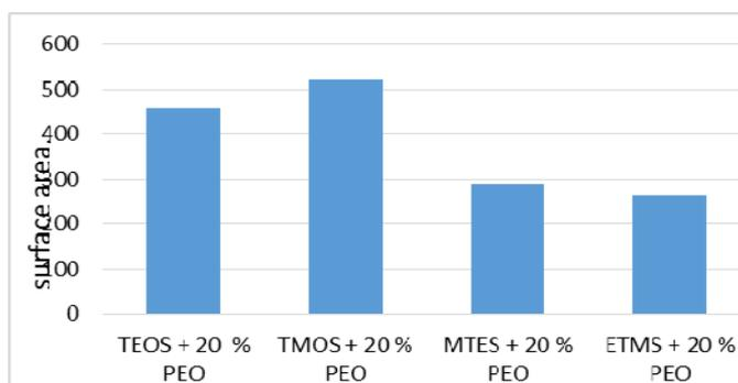
Fig.3. BET analysis of silica nanomaterials
