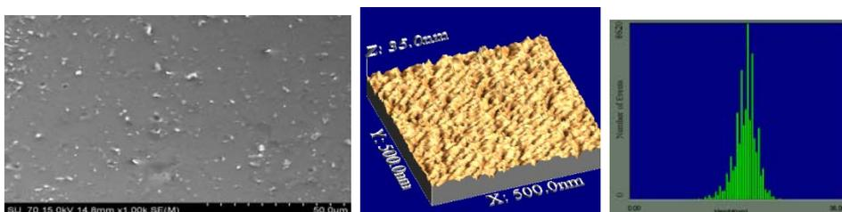
**Fig.7.** SEM, AFM image and roughness analysis of the hybrids with MTES containing 20 % PEO
