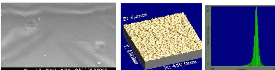
**Fig.5.** SEM, AFM image and roughness analysis of the hybrids with TMOS containing 20 % PEO
