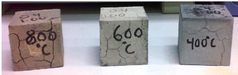
Fig. 5. The optimum Fly ash-based geopolymers with optimum compressive strength of 8.61 MPa, Fly Ash/Activator ratio= 2.0 and  $\text{Na}_2\text{SiO}_3/\text{NaOH}$  ratio = 2.5, after heat treatment at 400°C, 600°C, and 800°C
