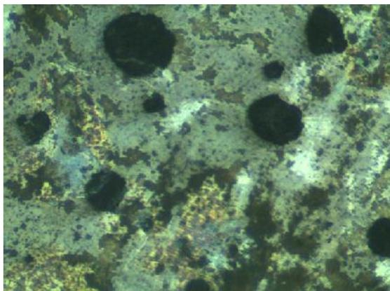
**Fig.3.** Optical metallography, X200. Nodular graphite pearlitic-ferrite matrix.
