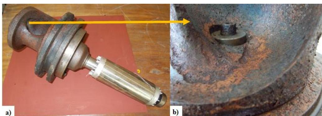
**Fig.2.** One-channel centrifugal pump for low pressure; a) impeller; b) corrosion wear zone of impeller.
