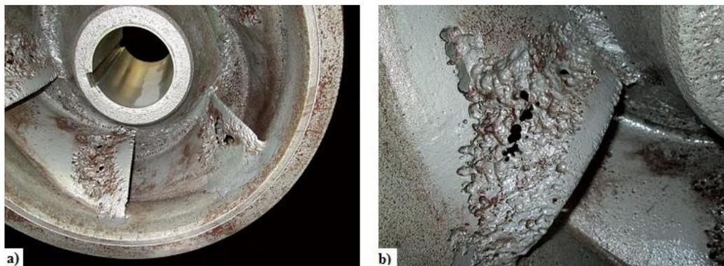
**Fig. 1.** Images of some used pump impellers: a) Cavitation wear; b) Detail.
