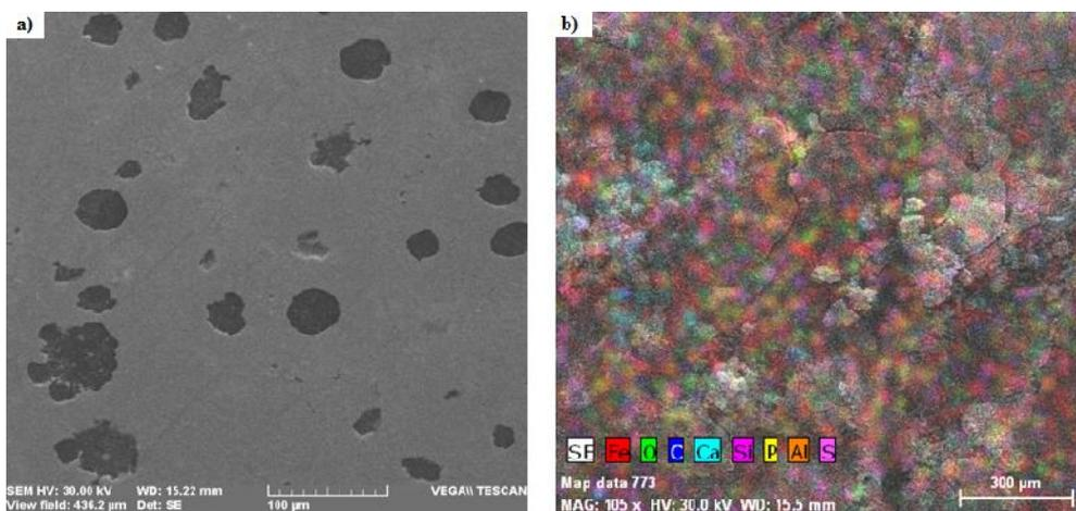
**Fig. 4.** The microstructure obtained with the Scanning electron microscope of the pump impeller: a) SEM microstructure, 100 µm; b) EDX microstructure, 300 µm.
