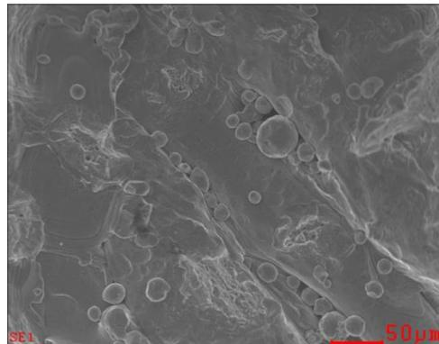
Fig. 6. Tensile fracture (energy density, 1.67 J/mm<sup>2</sup>) surface showing unmelted particles and partial fusion
