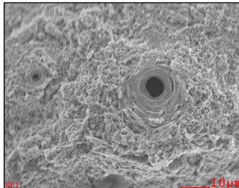
**Fig. 8.** Tensile fracture (energy density, 3.75 J/mm<sup>2</sup>) surface revealing a highly ductile fracture features with voids
