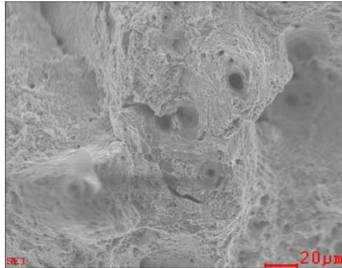
**Fig. 7.** Tensile fracture (energy density, 2.0 J/mm<sup>2</sup>) surface showing honey comb structure and cleavage features at isolated locations
