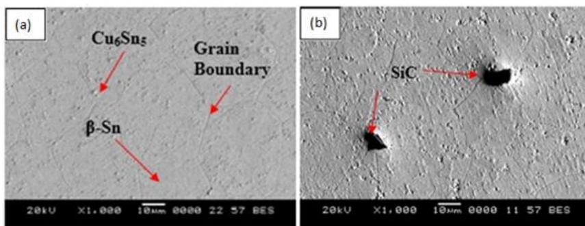
**Fig. 2.** SEM microstructures of; (a) pure SAC solder; (b) SAC-0.25SiC composite solder.
