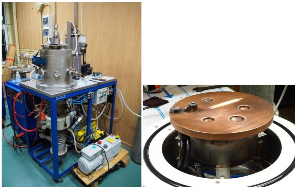
**Fig. 1.** Vacuum arc furnace
