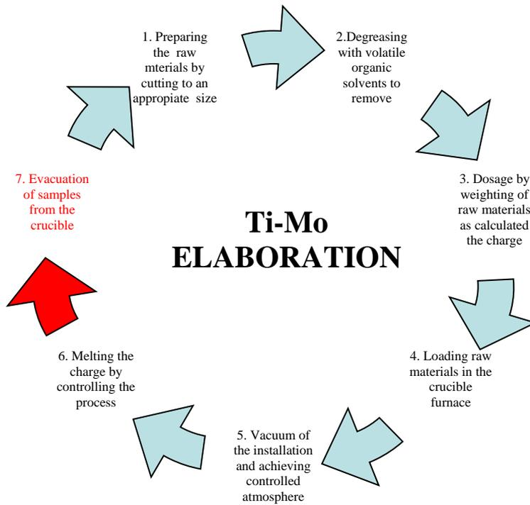
**Fig. 2.** Technological flow of Ti-Mo alloys
