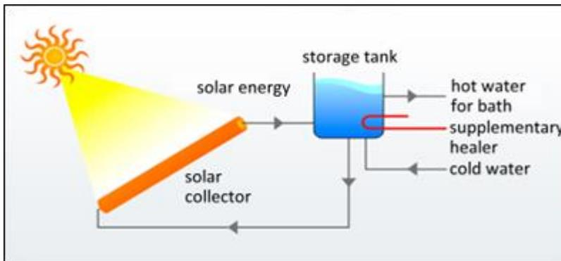
Fig. 1. natural circulation system of solar water heater [8]
