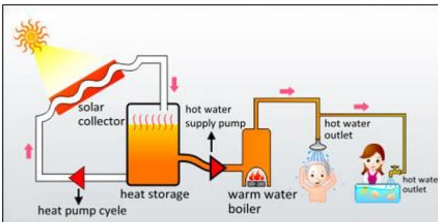
Fig. 2. Forced Cycle type of Solar water Heater [8]
