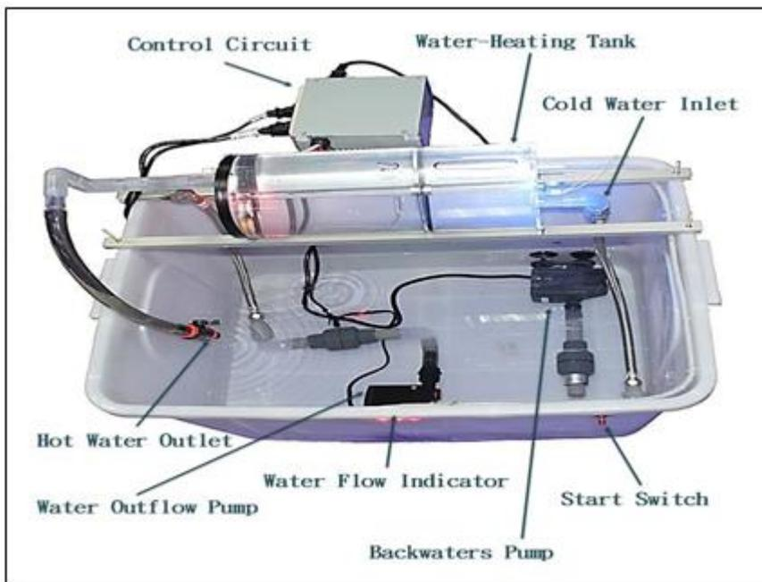
Fig. 6. Model of solar water heating tank
