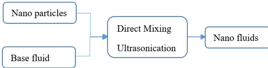
Fig. 1. Illustration of the Nano-fluid
