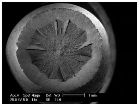
**Fig. 8.** Ductile fracture showing the typical cup-cone geometry at CK35 steel after quenching and tempering
