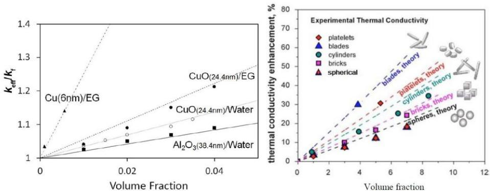
Fig. 2. Thermal conductivity enhancement as a function of volume fraction of particles [10]:
