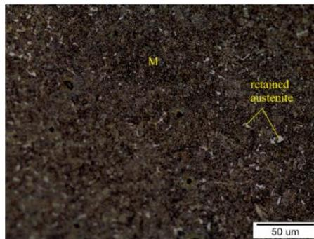
Fig. 6. Optical micrograph of microstructure of CK35 after quenching at nano-fluid water and tempering.
