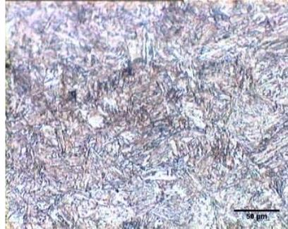
**Fig. 7.** Optical micrograph of microstructure of CK35 after quenching at water and tempering
