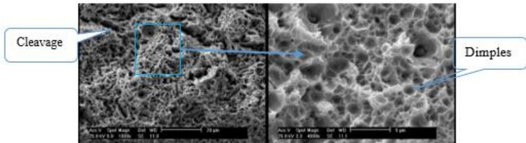
Fig. 10. Microvoids on the fracture surface of CK35 tensile test piece
