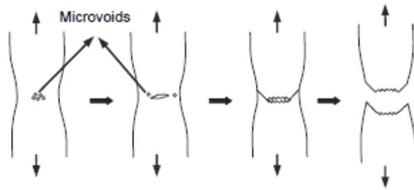
Fig. 9. Schematic representation of the cup-cone geometry formation during the ductile fracture process
