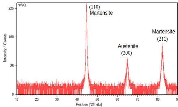
Fig. 5. X-ray diffraction profiles of CK53 after quenching at nano-fluid water and tempering.
