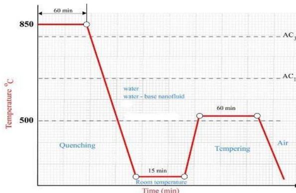
**Fig. 3.** Schematic illustration of heat treatment cycle used in this study.
